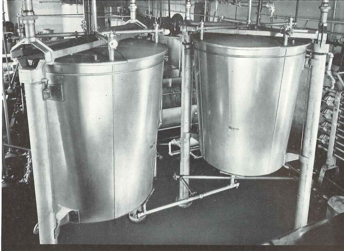
Two CP Milk Irradiators at Producer's Creamery, Benton Harbor, Michigan. All milk delivered by this progressive concern is irradiated.
