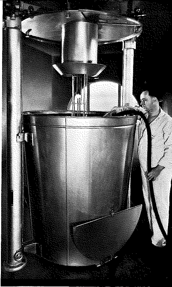
Cleaning the irradiator. Lowering drum permits reaching all surfaces coming in contact with milk.
